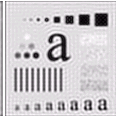
Result of filtering with ideal low pass filter of radius 30
